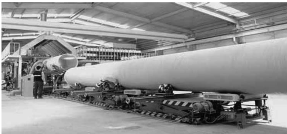
Figure 60. Continuous filament winding process.
