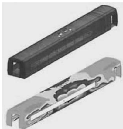
Figure 21. FE analysis to design and verify the structural safety of composite car body of Tilting Train eXpress (TTX).
