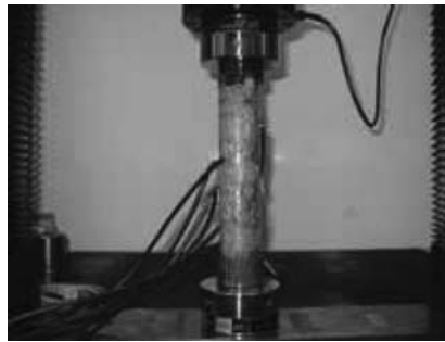
Figure 33. Compressive test for hybrid braid composite.
