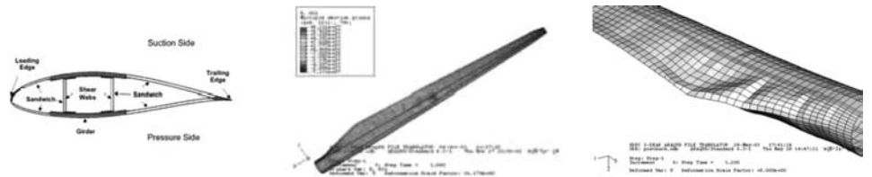
Figure 43. Rotor blade for wind turbine and its static/buckling analysis.
